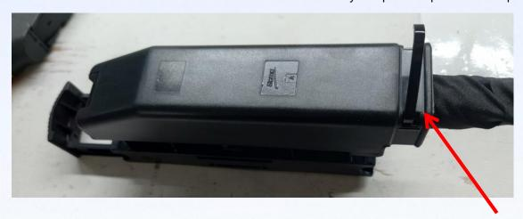
**Step 3:** Remove the protection cap by sliding to the front.
