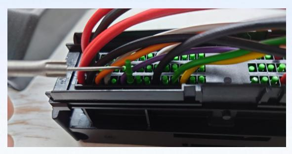
**Step 7**Install the contact with wire in cavity 67 and push until it is seated firmly. Test if the contact is firmly seated by pulling slightly on the wire. The wire should remain seated.
