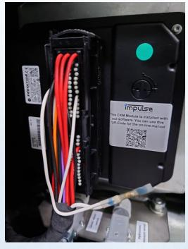
Fixate the wire with a ty-wrap or tape and re-install the protection cover. Install a ty-wrap around the protection cover to make sure that all wires have sufficient strain relief, and all wires are not harmed by potential mechanical stress.
