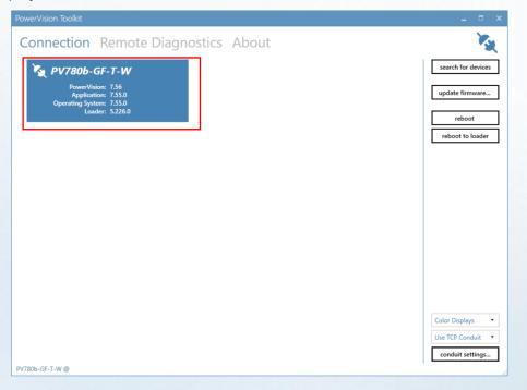
From this point, you can select "Remote Diagnostics" from the horizontal menu. At that moment, the pump screen comes forward and can be viewed remotely. When the screen is in sleep mode, a command can be sent via the menu option "Events". NB! It takes a few seconds to wake the screen from sleep mode.
