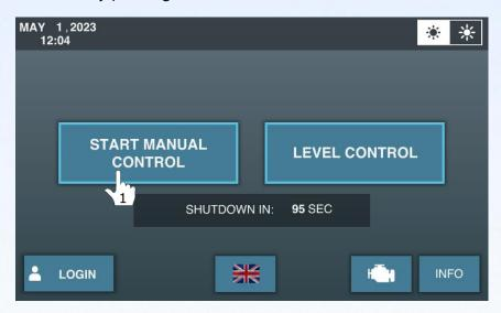
Be aware that RPM adjustment is only possible as soon as the system has been primed (full of water). As long as there is no water present, the REV UP and REV DOWN buttons are not being displayed on the screen.
