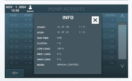
DIESEL PUMPS WILL SHOW THE PERCENTAGES OF LOAD REFERRED TO MAXIMUM ENGINE LOAD. A MINIMUM OF 40% ENGINE LOAD IS NEEDED FOR MODERN ENGINES TO KEEP THE EXHAUST AFTERTREATMENT SYSTEM IN ITS OPERATIONAL LIMITS. IF THE ENGINE LOAD IS TOO LOW A FAULT CODE WILL APPEAR!
