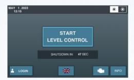
The **Level Control (Only)** software option is mostly used for larger pump sets for which Ecomizer-Pro can help reduce mistakes caused by human error.
