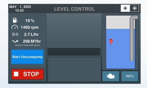
As long as the float switch is up the engine will slowly rev up to maximum RPM.
