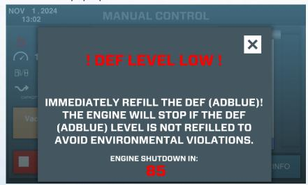
Once the DEF level low shutdown timer is finished the engine will be stopped and a fault code is added to the fault code list. Also, a notification pop-up will be shown that the engine has been stopped due to the neglected refueling of DEF.
