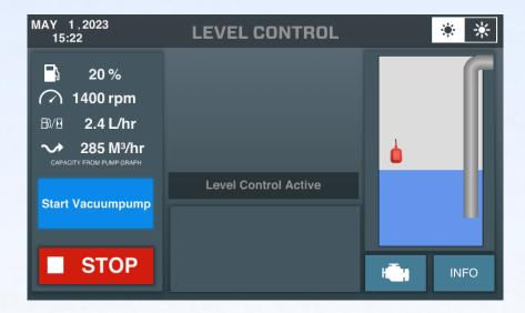
As soon as the water level comes up to a level that the float switch will come up again the pump will rev up again.
