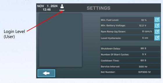
As User possibilities are given to shut down fuel tank levels (by running on an external fuel tank) and start on Ball Float Alarm Level (both sensors connected at the same time).
