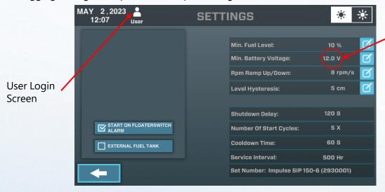
Battery voltage at which battery rechain will be activated.
