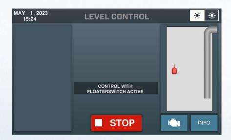
As soon as air enters the suction line the pump will shut itself off (stops) and will be waiting until the time the float switch will be up again.
