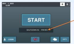
The pump will automatically shut down in Stand-By mode as soon as there are no further interactions with the display for more than 120 seconds.
