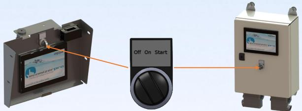
All Impulse Pumps equipped with ECOMIZER-PRO are operated using only a single switch. To activate the display, keep the switch in the "Start" position <u>until the display lights up</u> (approximately 5 seconds). Once it has lit up, you can release the switch, which will return to the "On" position. In the "On" position, the unit is active for remote operation.
