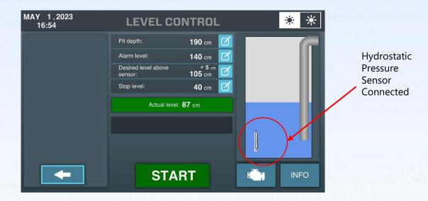
The HPS sensor should be positioned at the bottom or just above the bottom (to avoid sludge) of the pump pit. Make sure that the sensor is always leveled below the suction hose/strainer of the pump. The best way is to install the HSP inside a well point (filter tube) and as far away as possible from suction inlet/strainer.
