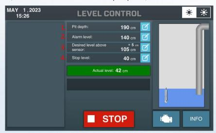
The parameters for level control can be set by pressing the blue activation box for the level that needs to be changed/adjusted.
