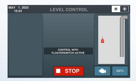
As soon as the water level will activate the pump by lifting the float switch up, the following screen appears:
