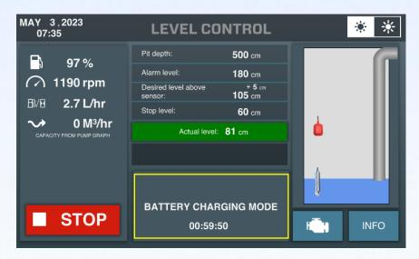
The Min. Battery Voltage can be adjusted in the settings menu which is visible after logging in. Login is explained in chapter 9 (Login User).
