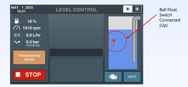
The vacuum pump is active and will prime the system. After full activation the following screen appears:
