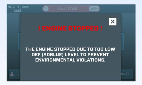
As long as there is no DEF added the engine can be started to show correct behavior of the control system but will always trigger the shutdown procedure after 2 minutes. Only after at least 25% DEF level has been noted the shutdown procedures won't be triggered.
