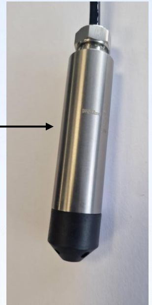
Filter/well-point tube. Placed at the bottom of the pit.
